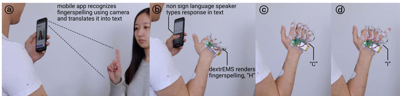
**Figure 13:** Our custom smartphone application detects fingerspelling by using MediaPipe and translates it into text. (b) The user types its response “HCI” onto the smartphone, which (b, c, and d) dextrEMS outputs by actuating the fingers to form a fingerspelled “HCI”.
