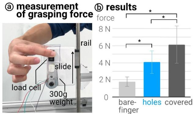
Figure 5: (a) Study apparatus of lift-and-hold task. (b) Force results for the grip task.
