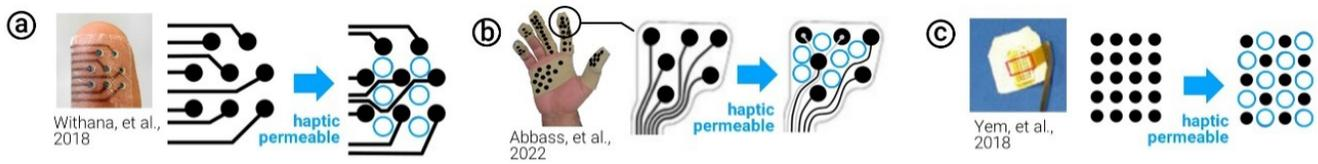
**Figure 10: Simulating the addition of holes (blue circles) to existing electro tactile devices. (a) [51]; (b) [1]; (c) [55].**
