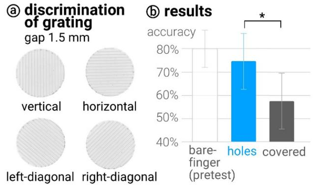
**Figure 4: (a) Tactile sensitivity task (grating orientation); (b) Results from tactile sensitivity task.**
