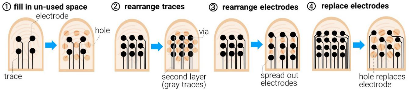
Figure 3: Four design options to implement haptic permeability on an electro-tactile device.
