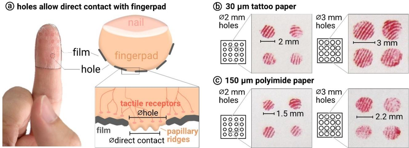
Figure 2: (a) Holes on the film allow direct contact with fingerpad, revealing papillary ridges and can directly transmit tactile signal to receptors. (b) Ink test on tattoo paper with holes. (c) Ink test on polyimide paper with holes.
