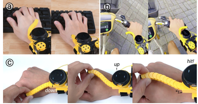
Figure 4: (a) The length of the tentacle represents the remaining time in a Pomodoro timer. (b) The tentacle's direction provides navigation cues. (c) The tentacle serves as a controller to play a Pong game with haptic feedback.
