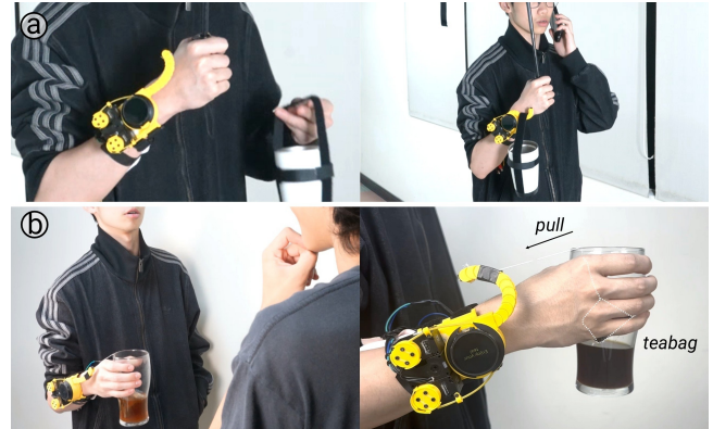
Figure 5: (a) The tentacle acts as an additional "finger" to hold a beverage when the user's hands are occupied. (b) The tentacle pulls out a tea bag when the timer is up.
