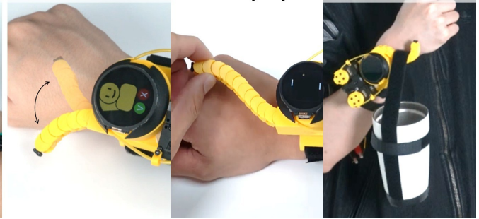
Figure 1: (a) We propose a novel actuator that is rolled under the smartwatch screen. The actuator, which is a custom tentacle actuator, can be extruded to variable length on demand and controlled through cable-driving motors. (b) The actuator can augment interactions for the smartwatch, e.g., extending the display for a phone call as a waving hand, extending the input for playing games, and for everyday life, e.g., helping hold a beverage when hands are occupied.
