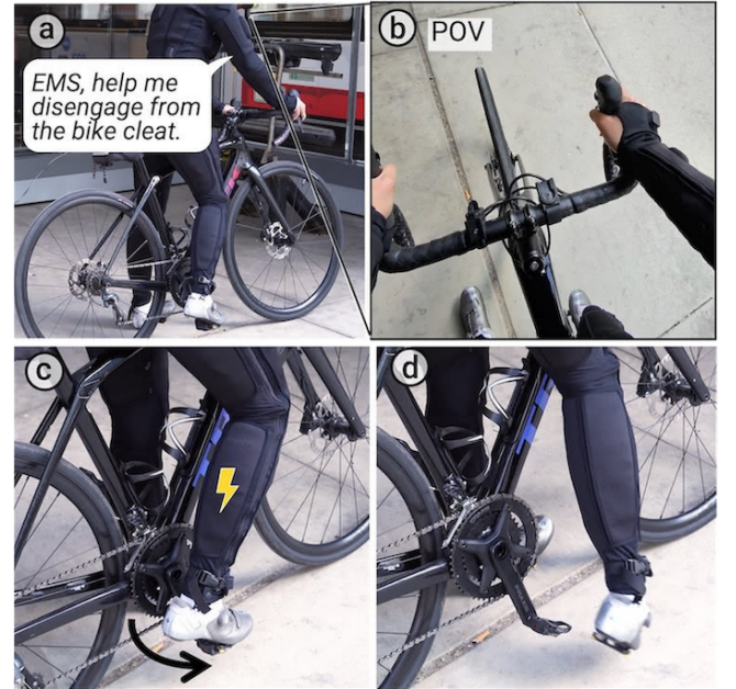
Figure 24: Our system uses (a) user’s spoken request; and (b) POV image, to (c) provide physical assistance through muscle stimulation of her heel, enabling this user to (d) successfully disengage from the bike pedal.
