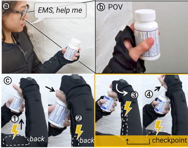
Figure 5: (a) User asks for help with a pill bottle. (b) Their POV. (c) The system can understand some degree of the state of objects, which is used to add “checkpoints” to the muscle-stimulation instructions, e.g., repeat until the cap is removed. (Although, as we will see in the next step of this walkthrough, this will not open this type of pill bottle.)
