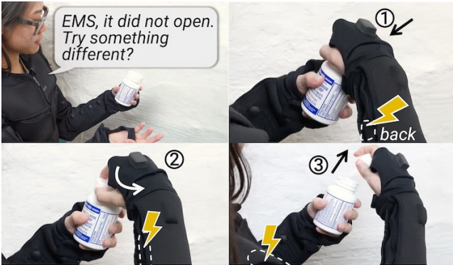
Figure 6: (a) User intervenes and asks for a different approach, which triggers our system to generate a new sequence of electrical muscle stimulation assistance.
