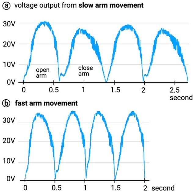
**Figure 15: Voltage (rectifier output) of our harvester for two consecutive elbow movements (flex/extend for each movement).**
