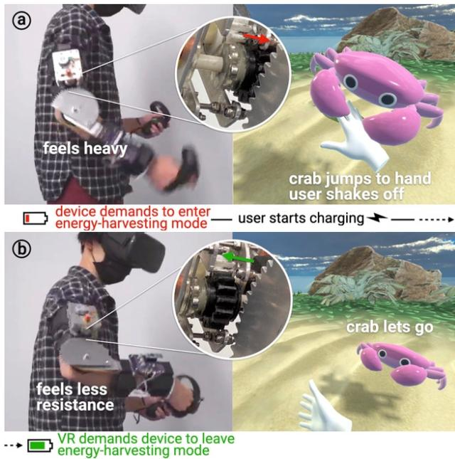
Figure 6: (a) The device senses low power, enters energy-harvesting mode, and informs the VR, which responds by rendering a crab jumping to the user’s hand. The user shakes off the crab by moving their arm, which charges the device, unknowingly. (b) When the device is charged, it leaves the energy-harvesting mode and informs the VR, which responds by rendering the crab let go.
