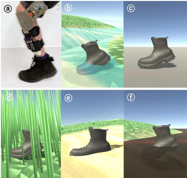
Figure 19: Our batteryless haptic device is worn on the foot in a VR running experience with haptic feedback.
