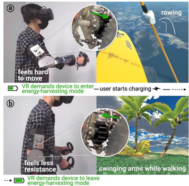
Figure 7: (a) VR demands resistive force (device enters energy-harvesting mode) for this rowing interaction; (b) VR demands leaving energy-harvesting mode after the user lands on another island to walk again.
