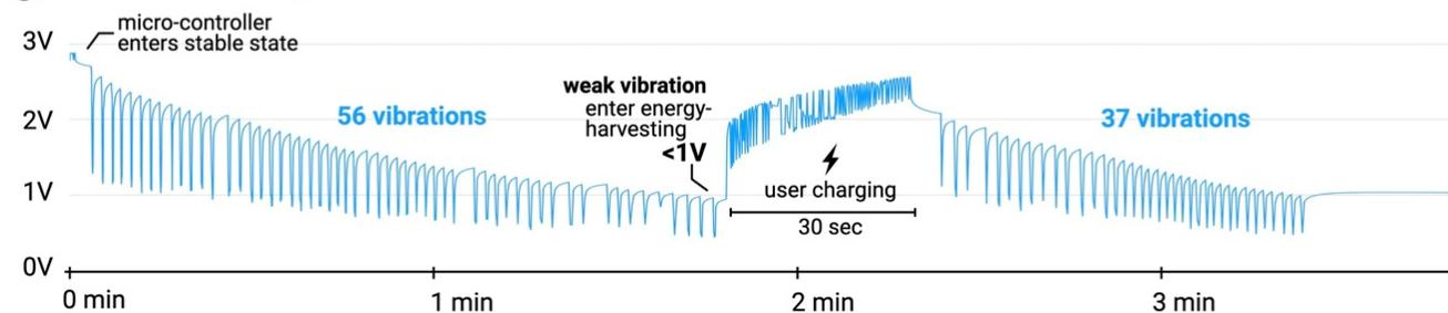
Figure 16: (a) Charging and discharging profile of our 0.33F supercapacitor used to power the haptic device’s microcontroller. (b) Charge/discharge profile of the two capacitors that switch our haptic device’s EPM clutch and the braking mode. (c) Charge/discharge profile of the capacitor used for electrical muscle stimulation, of 300ms in duration. (d) Charge/discharge profile of the super-capacitor used for vibrations, of 300ms in duration.
