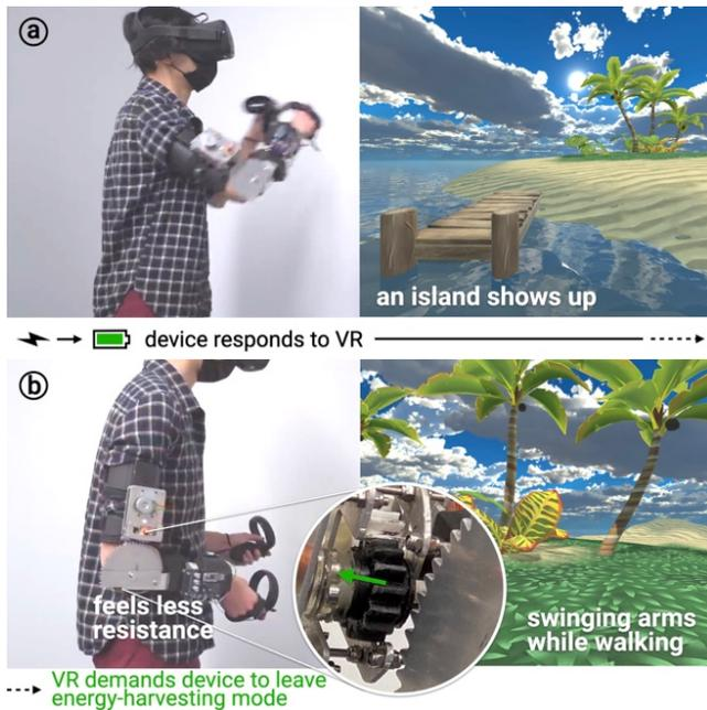
**Figure 4:** (a) The haptic device is now charged and responds to the VR of its charge capacity. The VR experience then renders an island. (b) The user walks on the island, so VR requests the device to stop harvesting mode: now the user’s arm feels less resistance.
