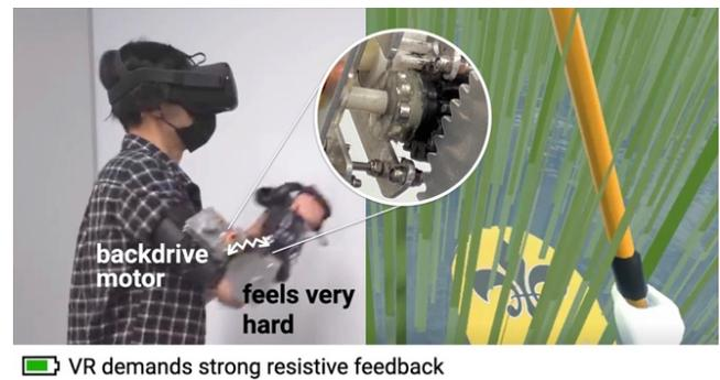
Figure 8: If there is a surplus of energy, the VR software launches one of the pre-made experience that can make use of this extra energy for a more immersive version of the current experiences. In this case, the user experiences paddling through dense reeds, which they experience a higher resistance as they paddle (which is achieved by braking the DC harvester itself).
