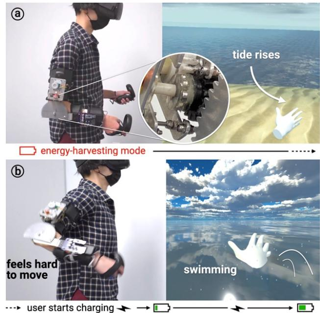
Figure 3: (a) When VR fails to connect to our batteryless haptic device, the VR assumes the device needs charging (and is in energy-harvesting mode) and renders a tide rising. (b) The user swims and feels resistance, *without even knowing they are charging the device.*
