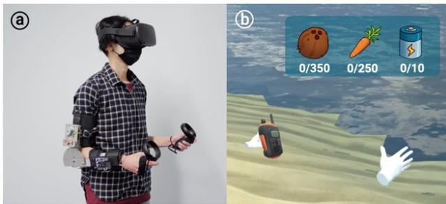
Figure 2: (a) A VR user with our batteryless haptic device worn on their arm. (b) At the start of our VR experience, the user finds themselves on a desert island. Their goal is to find water (coconuts), food (carrots), and batteries to radio call a rescue.
