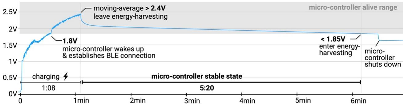
**(b) measuring harvesting for clutch operation & braking mode**
