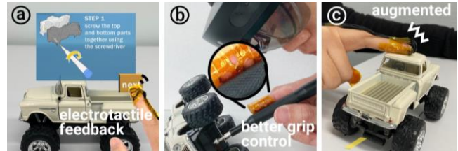
Figure 6: This approach enables dexterous activities in MR, where the user can feel haptic feedback for virtual interfaces (e.g., a button), can have better grip control when grasping physical objects (e.g., a screwdriver), and can experience haptic augmentation (e.g., vibration of a passive toy truck).
