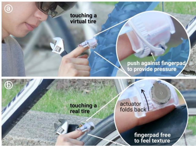
Figure 4: This approach enables a user in Mixed Reality to feel the texture of a virtual tire; yet they are also able to feel the texture of a real tire when they touch it, because the device folds back and reveals the whole fingerpad.
