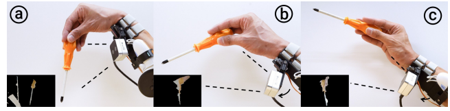
Figure 3: The wrist mount adjusts its view based on the pose of the hand, from (a) almost flat, (b) tilted, to (c) upright.
