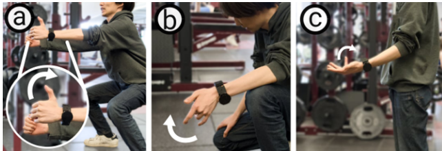
Figure 13: Not just for tracking fitness, a smartwatch can now physically support workouts with our wrist-EMS.
